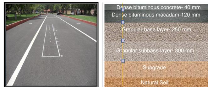
Figure 2: Crust composition of pavement
