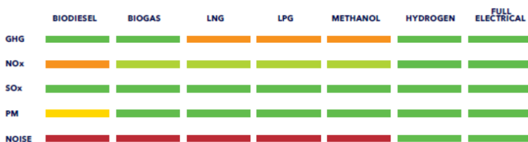
Figure 5-3 Diverse fuels and technologies differ in their potential to reduce various components of tank-to-propeller emissions from ships. The reductions illustrated are relative to using traditional fuels (HFO/MGO) (DNV GL 2018a). Green indicates high potential. Red indicates low potential.
